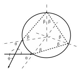
Defining the total angle  $\phi$  through which the light ray is refracted in the usual positive sense - i.e. counter-clockwise - then we have
