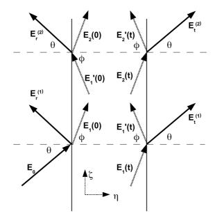
two prisms. The first two sets of reflection-refractions are shown in the figure. Note that by Snell's law, the angle of the transmitted wave is also  $\theta$ .
