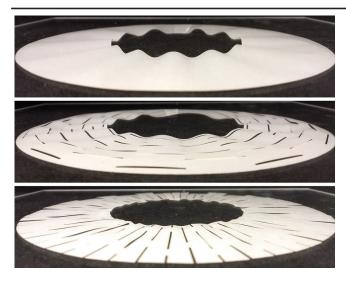
FIG. 4. (a) A conical annulus flattened under a piece of acrylic, with a small gap allowing for wrinkle formation. (b) Azimuthal slits do not affect the pattern of wrinkles. (c) Radial slits result in azimuthal quadrupoles, minimizing interaction energy with the curvature monopole. When flattened, radial slits lead to a soft response with no wrinkles.
