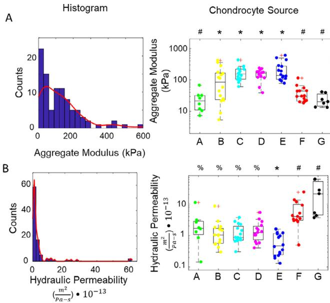
**Fig. 2.** Compressive properties summary: A) Aggregate modulus histogram shows a broad peak with right skewed data and a large range of values. B) Hydraulic Permeability histograms show a narrow peak with right skewed data and a large range of values. The chondrocyte source had a large effect on the hydraulic permeability and aggregate modulus. Different symbols indicate statistical significance ( $p < 0.05$ ).
