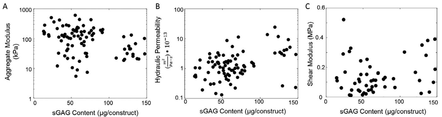
**Fig. 8.** The global structure function relationship of human tissue engineered cartilage showed no strong correlations between the global sGAG content and the A) aggregate modulus, B) hydraulic permeability, or C) the shear modulus. This lack of correlation may be caused by heterogeneity in new matrix deposition.
