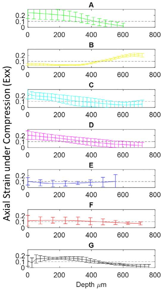
**Fig. 5.** Depth dependent axial strain for each chondrocyte source. Some chondrocyte sources produced uniform strain fields across the sample while other sources produced very heterogeneous strain. Gray dashed line is the input strain (10%).
