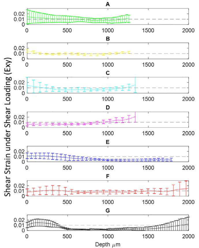
**Fig. 6.** Depth dependent shear strain for each chondrocyte source. Some chondrocyte sources produced uniform strain fields across the sample while other sources produced very heterogeneous strain. Additionally, the total length of each construct could vary based on the location of new matrix deposition. Gray dashed line is the input shear strain (1%).
