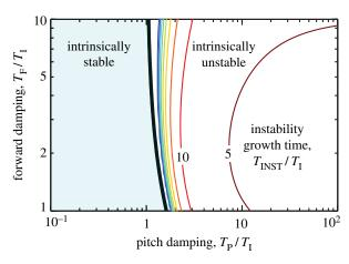
**Figure 4.** Stability diagram for insect flight. Stability characteristics are plotted as a function of dimensionless forward and pitch damping time scales,  $T_F/T_I$  and  $T_P/T_I$ . The light blue region to the left of the black line corresponds to intrinsic stability. The region to the right is unstable, and the contours show the dimensionless instability growth time,  $T_{INST}/T_I$ . (Online version in colour.)
