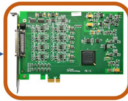
Data acquisition device
